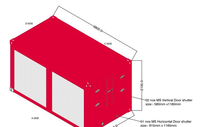
NOTE :- DIMENSION TOLERANCE  $\pm 20$  MM UPTO 500MM &  $\pm$  30 MM ABOVE 500 MM
